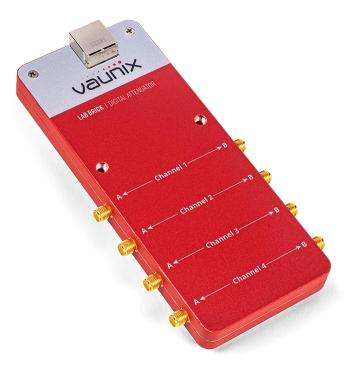
The Lab Brick LDA series of Digital Attenuators bring affordability, functionality, reliability, and simplicity to the microwave test bench. The LDA products range from 6 MHz to 40 GHz with input level tolerance to 2 Watts and step size as small as 0.1 dB.
