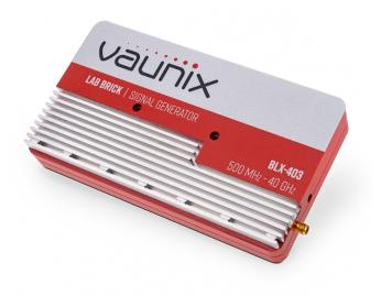
The Lab Brick<sup>™</sup> series of synthesized signal generators bring affordability, functionality, and simplicity to the microwave test bench. Vaunix offers standard products with frequencies covering from .5 MHz up to 40 GHz with 100 Hz frequency resolution, +10 dBm output power with a minimum of 40 dB output level control. They offer advanced features such as frequency sweeping, internal/external 10 MHz reference and standard pulse modulation.
